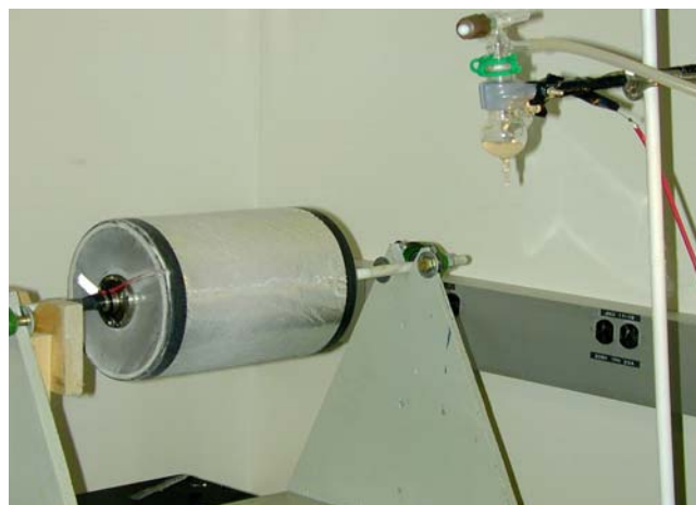
Fig. 2. Laboratory set up for electrospinning.
